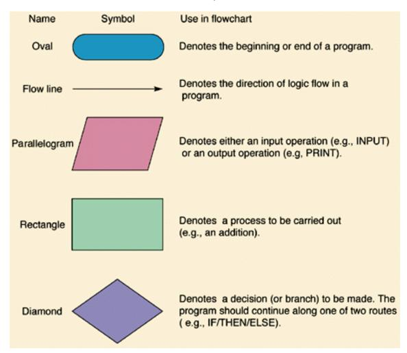
Flowchart is made up of the following logic structure,
